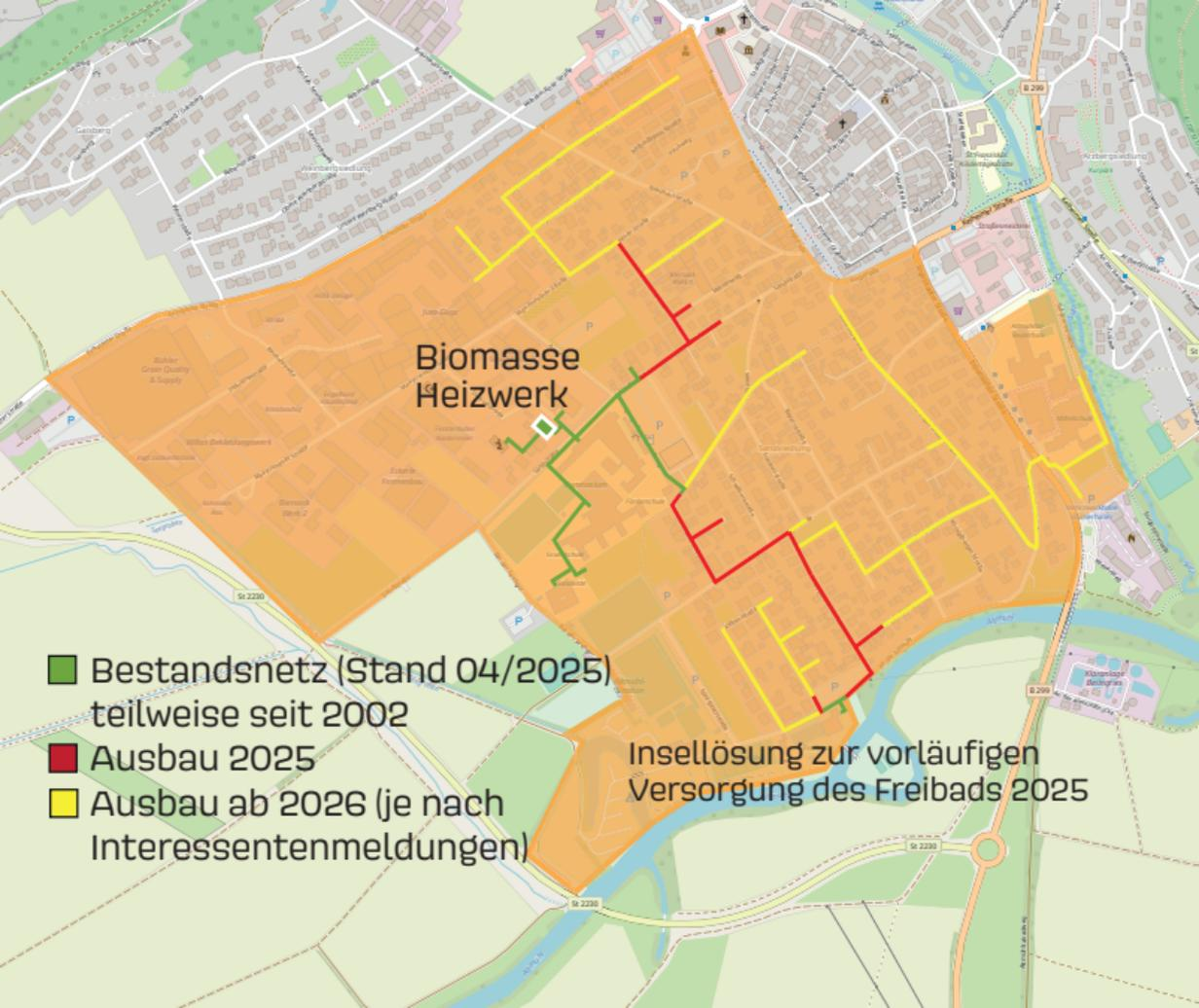
The map shows a residential area with a central orange-shaded region labeled 'Biomasse Heizwerk'. A network of lines is overlaid on the map, color-coded to show different stages of expansion: green for existing infrastructure, red for 2025 expansion, and yellow for expansion starting in 2026. The map also shows surrounding streets, a river, and various landmarks.
